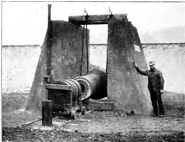
FIG. 94. Ballistic Pendulum (from Bureau of Mines Bulletin , No. 15)
